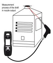
Put the probe of the KIGAZ 110 in the draft hood, going through the side openings of the boiler
