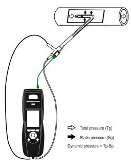
The Pitot tube must be introduced perpendicularly, in the middle into the duct and parallel to the flow.
