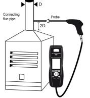
Put the probe of the KIGAZ 110 in the draft hood, going through the front face of the boiler
