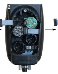
Disconnection of the ribbon cable of the sensor to replace Sensor rotation
